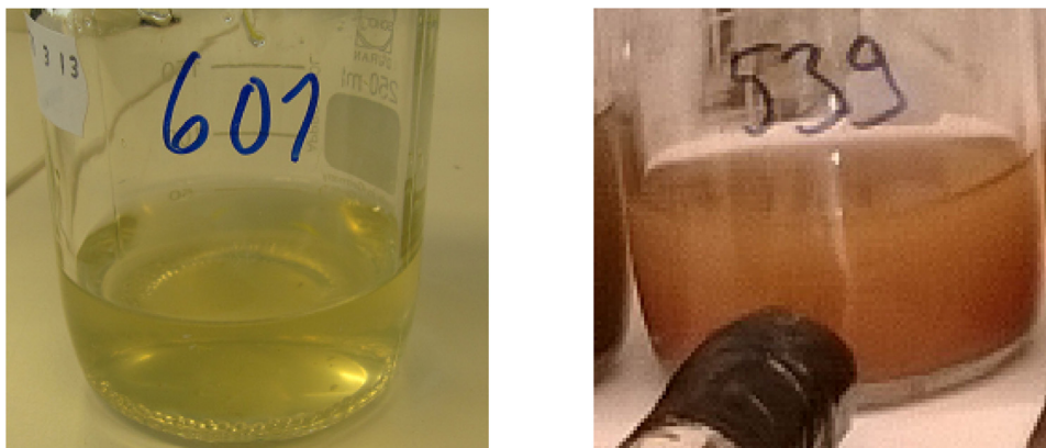
Fig. 8. Photographs representing different kind interactions between drinking water and pipe material. On left water sample from hot water circulation pipe after 5 min shaking with silica balls before installation of MWT and on right similar water sample after one year use of MWT.
