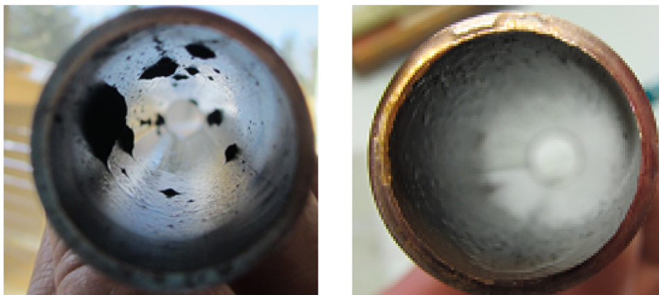
Fig. 7. Photographs showing the inside of the pipe. On left pipe sample from the hot water circulation before installation of MWT and on right pipe sample after one year of use.
